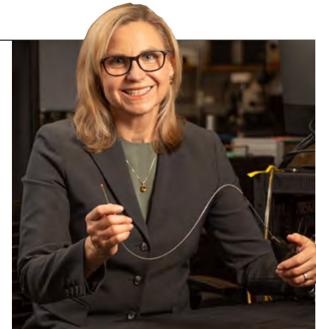
Jennifer Barton holds the falloscope, a sub-mm diameter endoscope capable of imaging the fallopian tubes. The device contains multispectral fluorescence imaging and optical coherence tomography, with the goal of early detection of ovarian cancer. Credit: Deanna Sanchez, University of Arizona.
