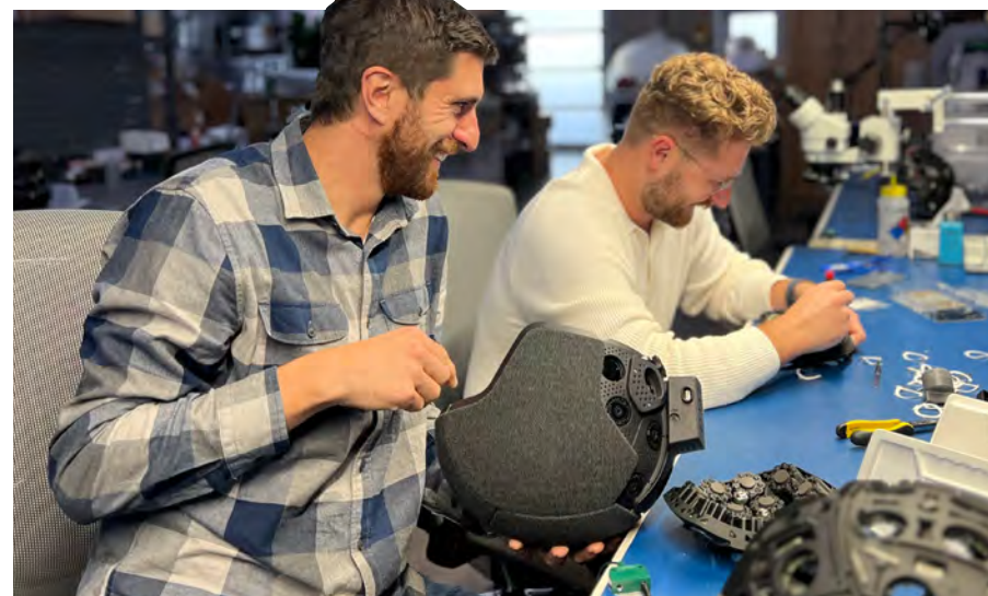
Ryan Field , left, in the lab working with the novel Flow2 helmet, which provides a uniform image of functional brain activity across the entire head. Credit: Kernel.
