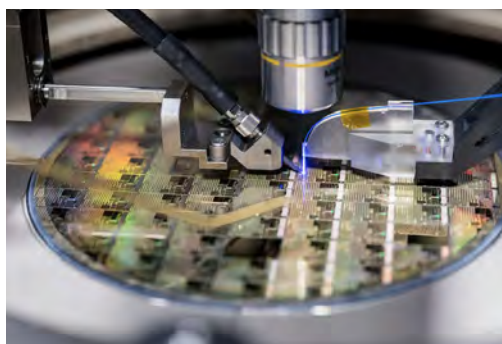
Electro-optical characterization of a microLED at wafer level. Credit: CEA-Leti.
