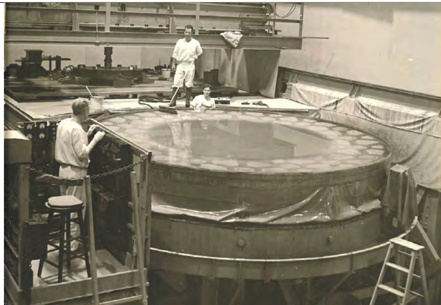
Stefan Sydor and others polishing the 200 inch primary for the Mt. Palomar Observatory. Credit: Sydor Optics.
