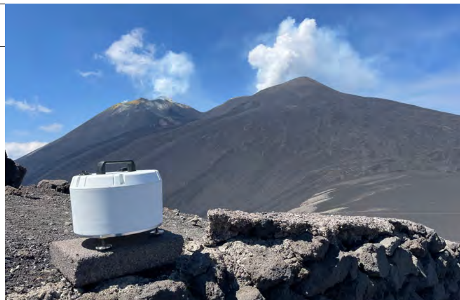
The “Wee-g” is said to be the world’s most sensitive MEMS gravimeter. Panel speaker Abhinav Prasad has taken this sensor from the lab to Mount Etna, Italy, where an array of Wee-gs now track volcanic activity. Credit: Courtesy of Abhinav Prasad, University of Glasgow.
