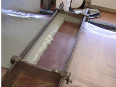
Figure 7.1, SMC Doctor Box Spreading Paste Layer on Carrier Film.
