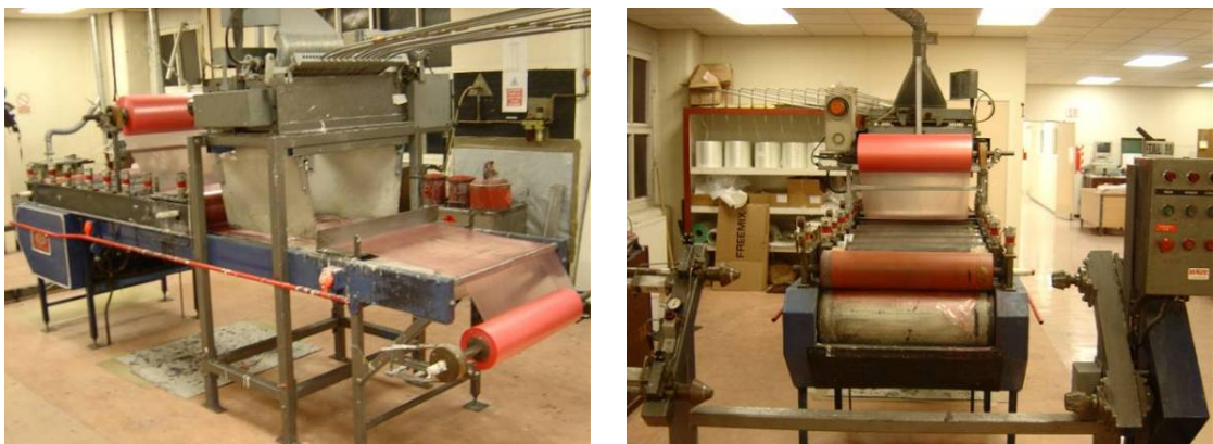
Figure 7.4, The SMC Pilot Production Line at Menzolit UK.
