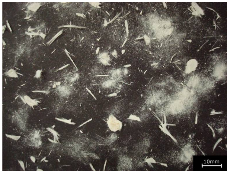
Figure 4.3, Recyclate Produced with an 8 mm Classifier Screen Aperture.
