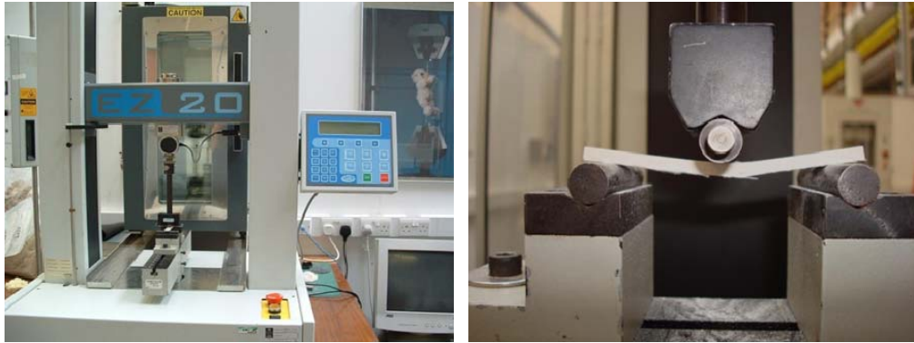
Figure 3.6, Three-Point Testing Equipment and Sample Set-up.
