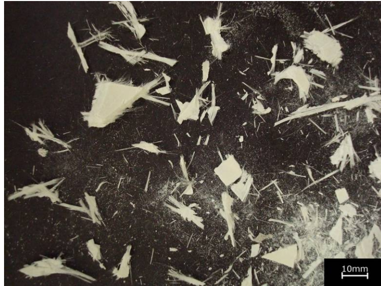
Figure 4.4, Recyclate Produced with a 10 mm Classifier Screen Aperture.
