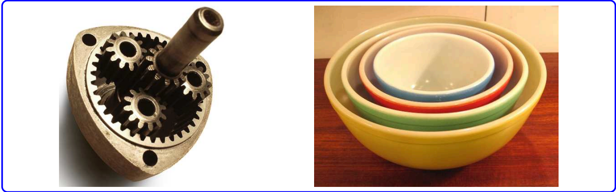
Figure 5.1: Two design examples (one from the engineering domain and one from product design) that are based on the same principle, namely the nested doll principle: Objects are contained in similar other objects in order to satisfy certain constraints. The left image is taken from http://en.wikipedia.org/wiki/Planetary_gears which is licensed under the terms of the GNU Free Documentation License. The image to the right is a set of “Pyrex Nesting Bowls”, found at http://www.whitetrashnyc.com/products/set-of-pyrex-nesting-bowls/1780 .
