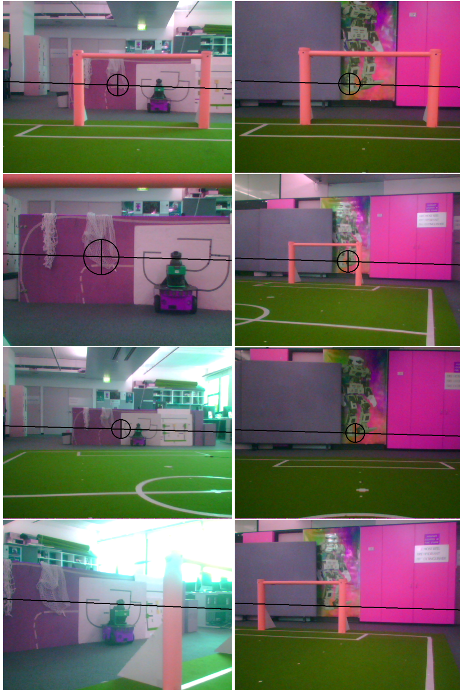
Fig. 7. Top row: Stored images of the left-hand and right-hand goal areas respectively. Row 2: Examples of correctly matched field views. Markers indicate the scale and position of the match. Row 3: Examples of correctly matched views with goals removed and overhead lights turned off. Bottom row: Some field views that could not be confidently matched to the stored images, possibly due to overexposure and occlusion of key features respectively.
