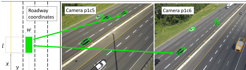
Figure 2: Example single annotation. The annotation is stored in roadway coordinates (left) but can be projected into cameras 5 and 6 on pole 1 (p1c5 and p1c6).
