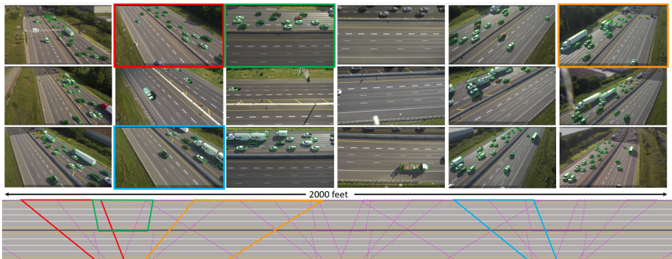
Figure 1: Example annotated (green boxes) frames from each camera field of view for one scene of the I24-3D Dataset. The approximate field of view for each camera is shown on the overhead roadway diagram below (some cameras shown in unique colors as examples). Regions outside of the considered field of view for each camera are blurred for this visualization. Cameras provide coverage of 2000 feet of Interstate-24 near Nashville, TN.
