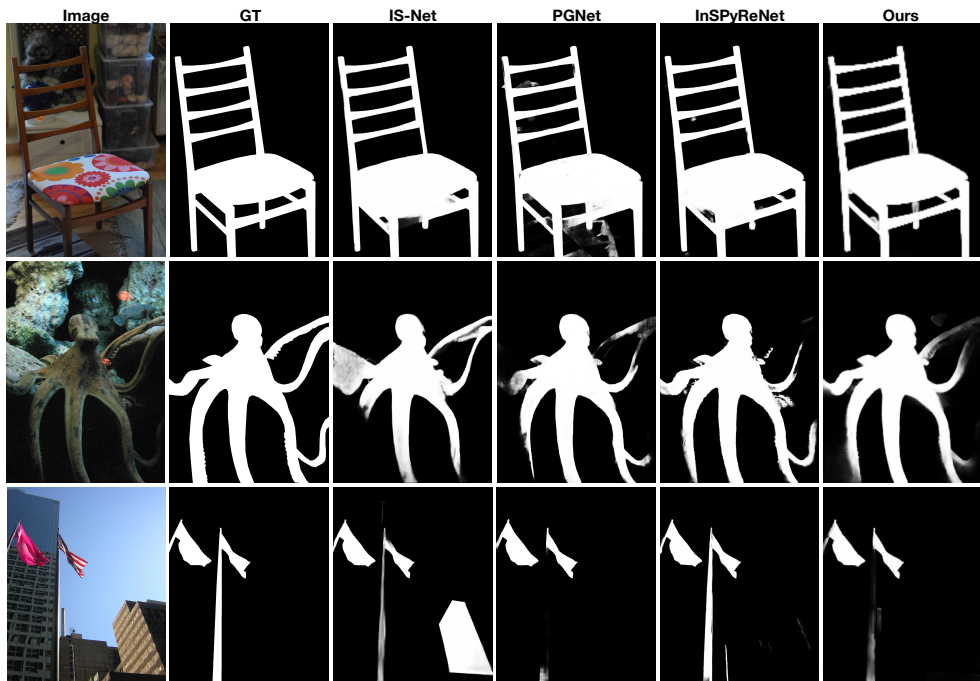
Figure 3: Qualitative comparison with the state-of-the-art methods on DIS5K dataset. Our proposed method is capable of capturing finer object details, such as chair legs and octopus legs. However, it may struggle in cases where an object has a reflection and is closely aligned to another object, such as the flagpole in the third row. Though InSPyReNet[20] predicts the contour of the flagpole, it also segments the pipe object in the building behind it.
