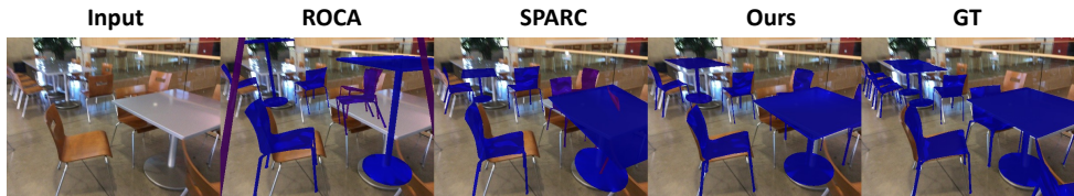
Figure 1: State-of-the-art methods for CAD model alignment from a single image. Using normalised object coordinates ROCA’s [14] alignments suffer from constant offsets. SPARC [23] produces more accurate alignments, but predicts CAD model poses individually which is slow and leads to worse predictions. In our method CAD model alignments are predicted jointly which is faster and more accurate.
