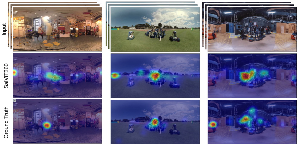
Figure 5: Failure cases. First column: Although SalViT360 detects the saliency of two men in the scene, it predicts a higher saliency for the drawing on the wall. Second column: Similarly, the model predicts false positives for the text added to the video later. Third column: When multiple people with similar visual attributes are located along the equator, the model tends to assign higher saliency near the centre due to the centre bias encountered in the ground truth fixations.
