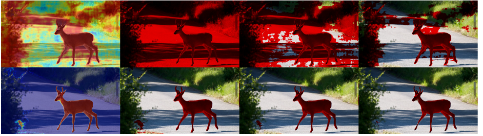
Figure 3: Comparison of Max. Entropy [8] (top) with Maskomaly (bottom) on an image from SMIYC [9]. The first column shows dense predictions; the others show predictions thresholded at 0.3, 0.5, and 0.8. ME achieves 95.5% AP and Maskomaly 98.9%.
