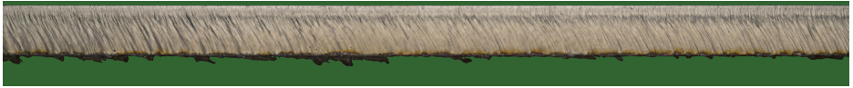
(a) Region of interest within an image showing the cut edge of a thermal processed sheet.
