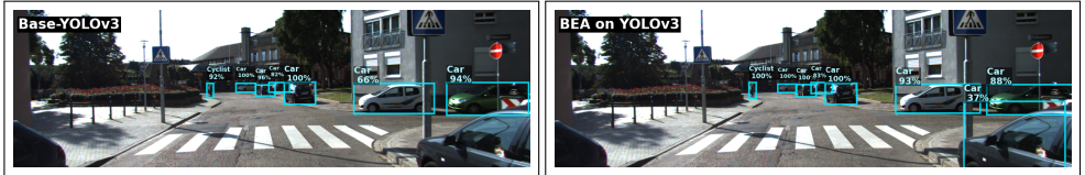
Figure 1: The figure on the left demonstrates uncalibrated confidence scores of Base-YOLOv3, where the white car has a 66% confidence score despite negligible occlusion, and the green car on the right edge has a 94% confidence score despite occlusion. In contrast, the right figure shows that BEA-YOLOv3 detects a car on the bottom right edge, which Base-YOLOv3 misses, and has superior confidence score calibration, indicating the effectiveness of our approach over baseline (Base-YOLOv3).
