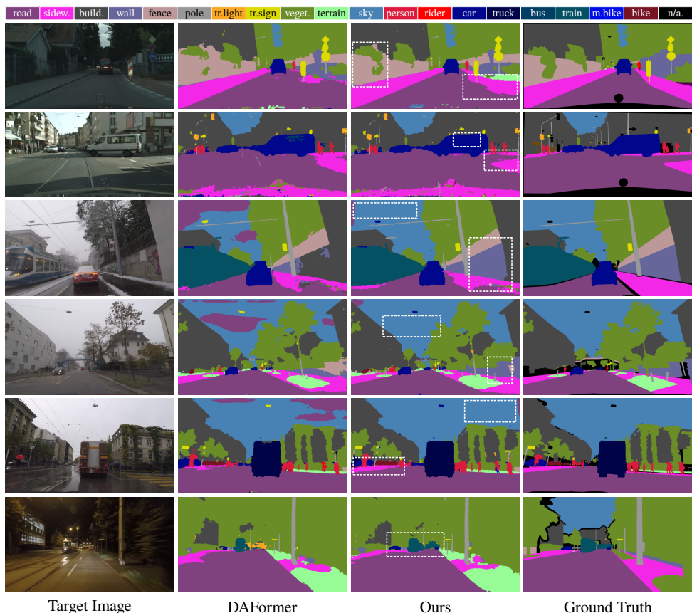
Figure 2: Qualitative semantic segmentation results of our method compared to the baseline DAFormer [10] on GTA→Cityscapes (row 1), SYNTHIA→Cityscapes (row 2), and Cityscapes→ACDC (rows 3-6). An extended analysis on example predictions is provided in the Supplementary Material.
