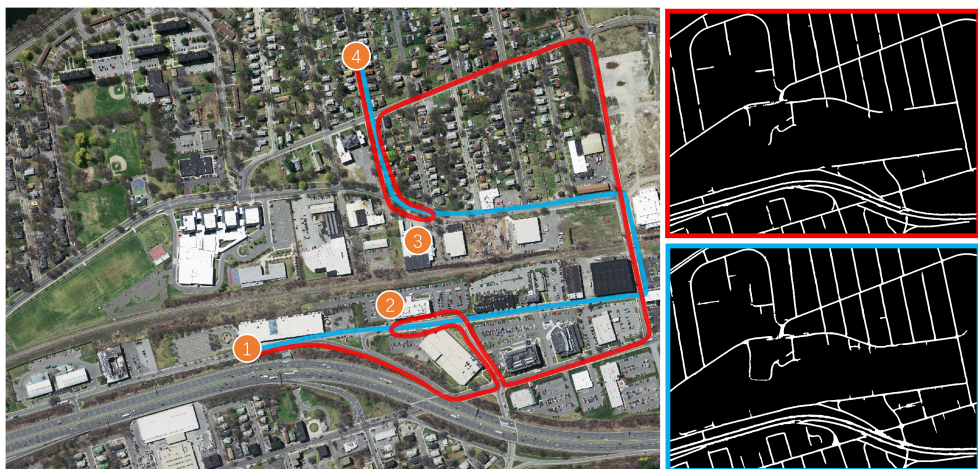
Figure 1: Significance of topological accuracy in road segmentation and subsequent route planning. The figure contains an aerial image from Massachusetts alongside two segmented road maps predicted by U-Net (top) [40] and ours (bottom), respectively. These two segmentation results achieve similar quality in per-pixel accuracy, but the top one is observed to have more broken roads. Road graphs are extracted from these segmentation [4] and further generate different optimal paths to visit the four locations in the image, which are depicted in red and blue, respectively. Bottom segmentation is evidently preferred, because the blue path is much shorter than the red one.
