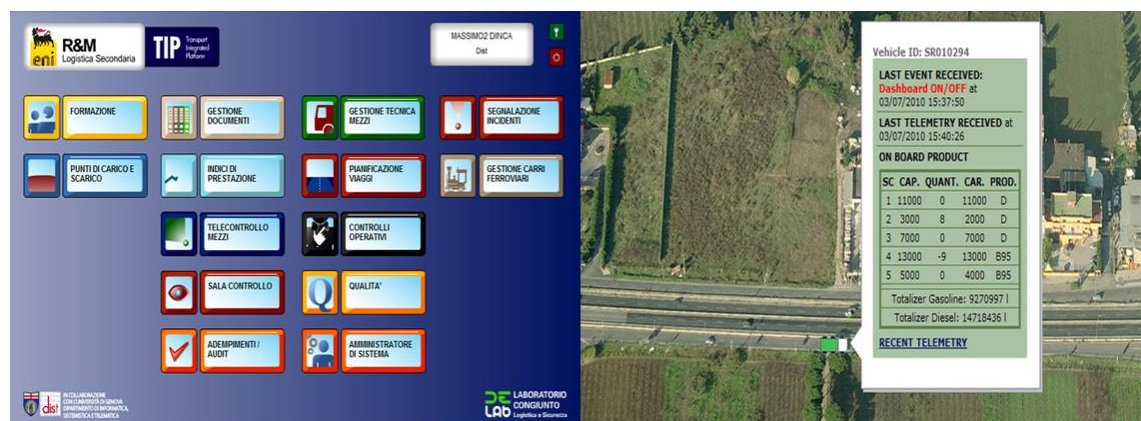
Fig. 1-6 The graphical user interface of the Transport Integrated Platform: the dashboard on the left, web mapping on the right showing a monitored truck over Italian territories.
