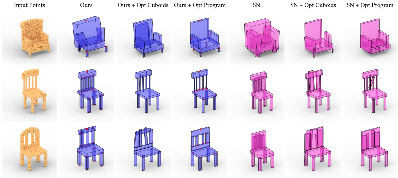
Fig. 13. Qualitative comparison of synthesis from point clouds of our method against StructureNet (SN). Our method is able to infer good program structures that match well with the unstructured geometry. The continuous parameters of this program structure can be further refined through an optimization procedure in order to better fit to the target point cloud without creating artifacts.
