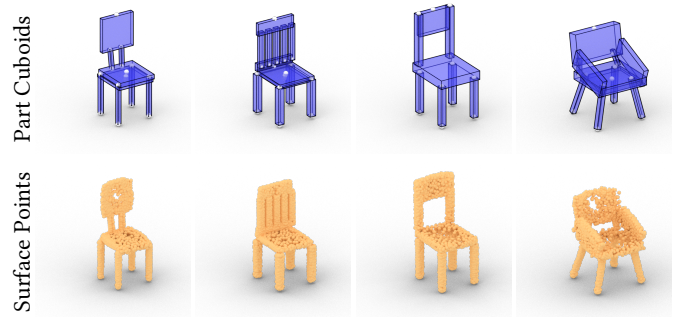
Fig. 12. Converting generated SHAPEASSEMBLY programs into dense point clouds. We use a point cloud decoder to predict the surface geometry of each leaf part proxy in our 3D shape structure. In this process, geometric details begin to take form, at the cost of some artifacts. We discuss a method for improving this procedure in section 8.
