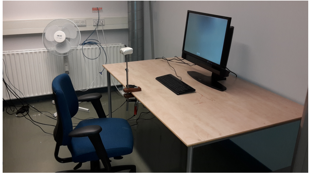
Figure 1 Experimental equipment: monitor with built-in eye tracker (SmartEye DR120), chin-rest, and keyboard.
