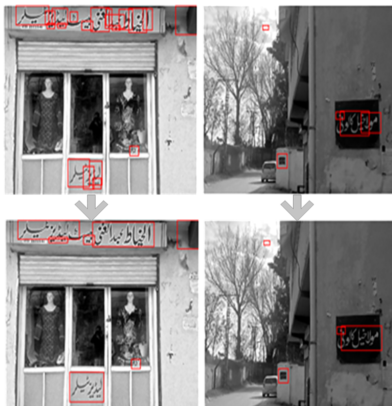
Figure 5 Text regions after SVM classification (top row). Candidate text regions fulfilling the criteria for text character linking are merged into text lines. Full-size DOI: 10.7717/peerj-cs.717/fig-5
