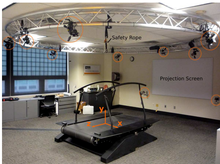
Figure 1. The treadmill with coordinate system, cameras (circled in orange), projection screen, and safety rope. The direction of travel is in the -z direction.
