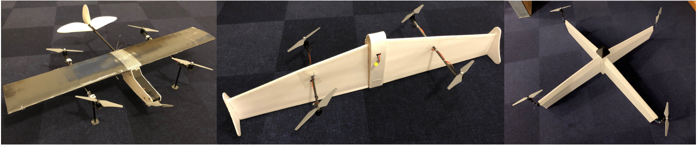
Fig. 6. The fabricated hybrid UAV models. From left to right: quad-plane (model 1), tail-sitter (model 2), x-wing (model 3).
