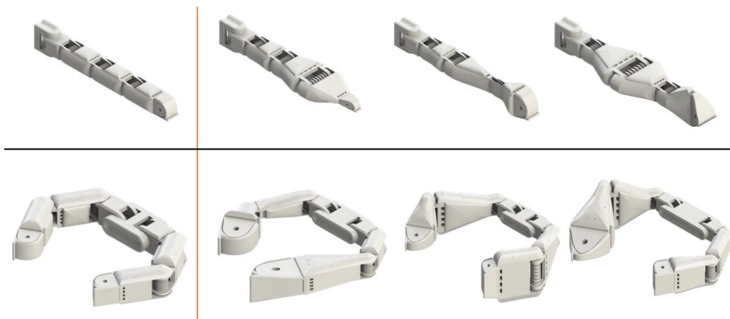
Figure 3-10: Morphology design space. The initial morphology of the single finger and the two-finger gripper designs are shown on the left. We randomly sample different parameters for each configuration and show the deformed morphology on the right.
