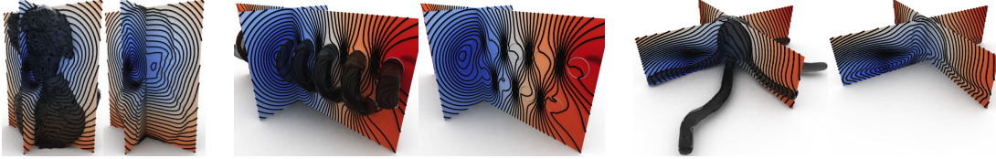
Figure 2.10: Examples of volumetric distances. The left image in each pair shows a surface (Beethoven bust, spiral, octopus resp.) cut by two planes; the right image shows the volumetric distance function on the two planes.
