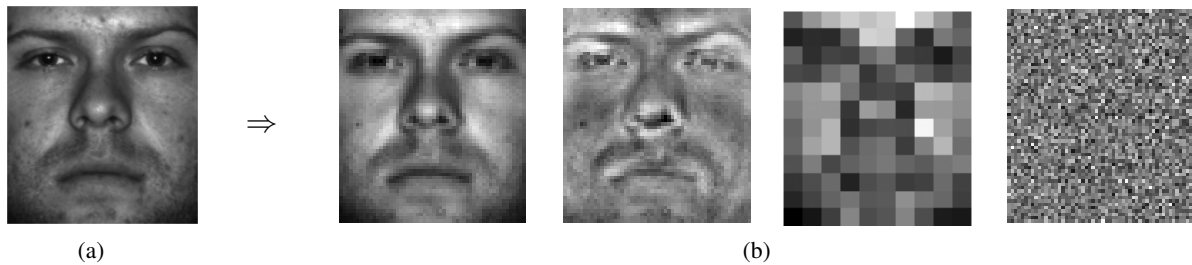
Fig. 1. (a). Original face image. (b). 120-D representations in terms of four different features (from left to right): Eigenfaces, Laplacianfaces, down-sampled ( 12 \times 10 pixel) image, and Randomfaces (see Section V for precise description). We will demonstrate that all these features contain almost the same information about the identity of the subject and give similarly good recognition performance.
