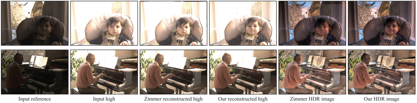
Figure 10: Comparison of our aligned reconstructions and HDR images with those of Zimmer et al. [2011]. Zimmer was given the input images to run their code on them directly. In this case, their method is not able to align the moving objects (e.g., the man’s reflection on the piano) which introduces ghosting in the final HDR image. Our method, on the other hand, produces better results.
