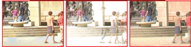
Figure 13: This scene from [Gallo et al. 2009] has moving people that sometimes appear in only one frame. We show the results of the deghosting methods of Gallo et al. (left) and Pece and Kautz [2010] (middle) using images provided by the respective authors. The former has block artifacts because of their per-block motion detection, and the latter still has some ghosting. Our method (top and right) can reconstruct the moving people, but it has artifacts as well. These appear as “washed out” regions where our algorithm only had information from one LDR image because the people in the reference disappeared in the other frames. Images courtesy of Orazio Gallo and Jan Kautz.
