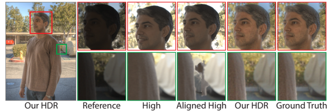
Fig. 2. We use the optical flow method of Liu [2009] to align the images with high and low exposures (only high is shown here) to the reference image. As shown in the top inset, optical flow methods are able to reasonably align the images where there are correspondences. However, in the regions with no correspondence (the bottom row), they produce artifacts. Our learning-based system is able to produce a high-quality HDR image by detecting these regions and excluding them from the final results.
