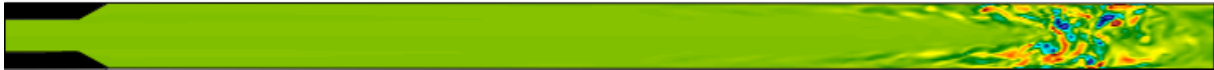
Figure 39. Numerical simulation results of the streamwise vorticity at Re = 2000 . The diverging angle is 45^\circ .
