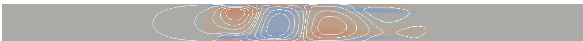
Figure 51. A snapshot of a simulation of the filtered Navier-Stokes equation. We use the plane Poiseuille flow with fixed flow rate. This is a spatially localized chaotic state, and we use this as a guess for a traveling-wave solution.
