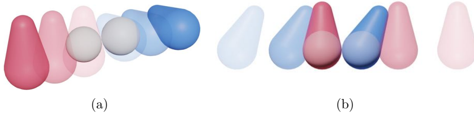
Figure 4: The trajectory of two medial primitives (using two medial cone as an example). The closer t is to t_0 , the higher the transparency of cones. The white spheres represent the contact sphere pair. (a) Condition 1: two cones are in contact at t_0 and separate away. (b) Condition 2: two cones are in contact at t_1 after passing through each other.
