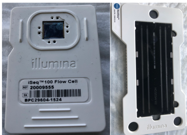
Fig. 3. Left: iSeq 100 flow cell. Right: NextSeq 500 Mid Flow Cell.
