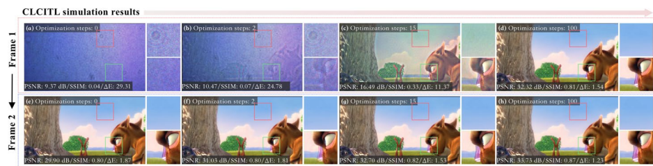
Fig. 7 Numerical simulation results of the CLCITL optimization. a-d The simulated results of the “Frame1”, most of the color and noise issues are addressed well. e-h The simulated results of “Frame2”, the reconstructed image is approach to the target image faster than that of “Frame1”. Images Credits: Big Buck Bunny, Blender Foundation [60]
