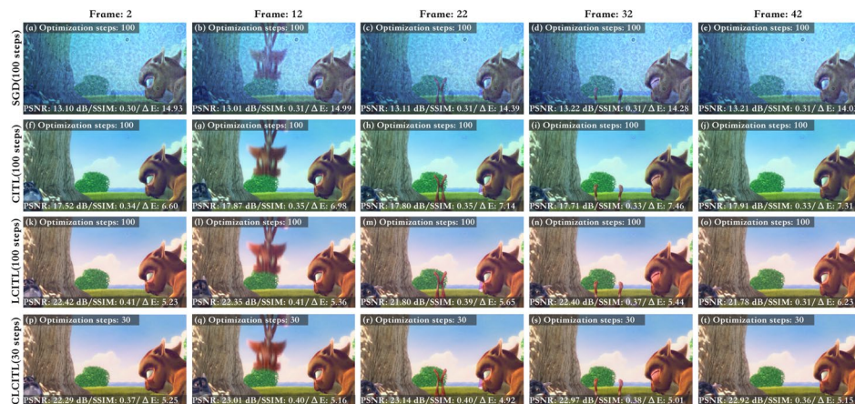
Fig. 13 Experimentally captured results with SGD, CITL, LCITL, and CLCITL method at different frames. Compared to the SGD method a-e , the CITL method f-j can eliminate most of the noises, while the color shift issue still exists in both methods. When we adopt the color-aware LCITL optimization k-o , both noise and color accuracy issues are addressed well. p-t The CLCITL method can significantly speed up the color-aware optimization while maintaining the similar image quality (see visualization 3 in supplementary material). Images Credits: Big Buck Bunny, Blender Foundation [60]
