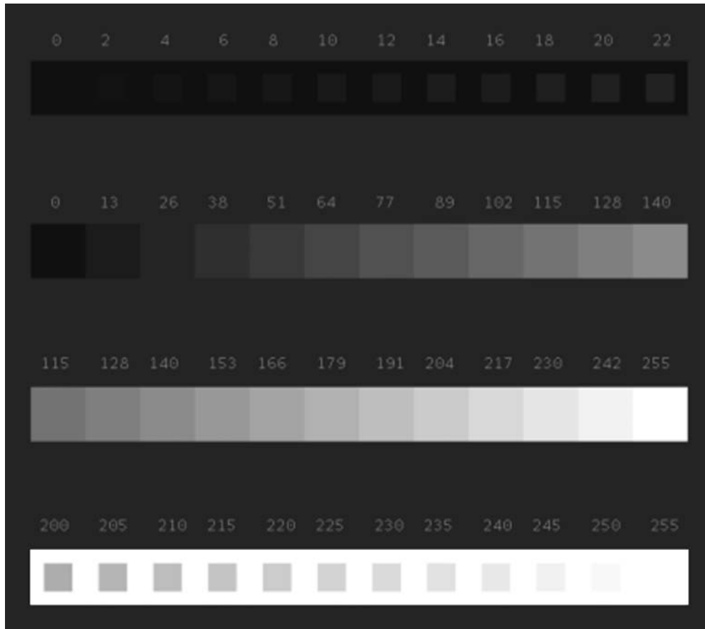
Fig 6. Quarterly display calibration test pattern.
