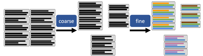
Fig. 2. Pipeline for InfoShield: Taking crawled ads as input, InfoShield-coarse groups these ads into micro-clusters, and InfoShield-fine highlights the common phrases in each ad by finding a common template.
