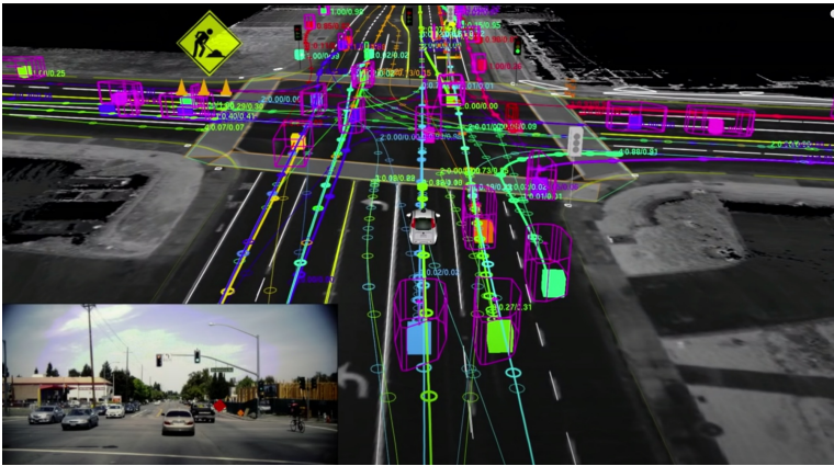
Figure 4.6: The output of perception modules for a typical autonomous vehicle (taken from https://www.youtube.com/watch?v=tiwVMrTLUWg ). The global occupancy grid is shown in gray (see the sides of the road). The local map is not shown in this picture but you can imagine that it has occupied voxels at all places where there are vehicles (purple boxes) and other stationary objects such as traffic light, nearby buildings etc. Typically, if we know that so and so voxel corresponds to a vehicle, we run an Extended Kalman Filter for that particular vehicle to estimate the voxels in the local map that it is likely to be in, in the next time-instant. The local map is a highly dynamic data structure that is rich in information necessary for planning trajectories of the robot.
