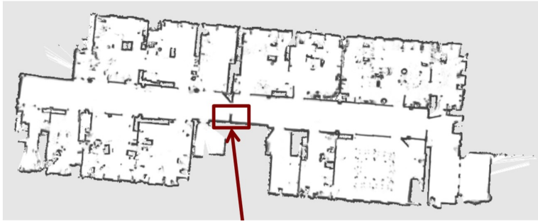
Figure 4.3: A grid map (also called an occupancy grid) is a large gray-scale image, each pixel represents a cell in the physical world. In this picture, cells that are occupied are colored black and empty cells represent free space. A grid map is a useful representation for a robot to localize in this house using observations from its sensors and comparing those to the map.
