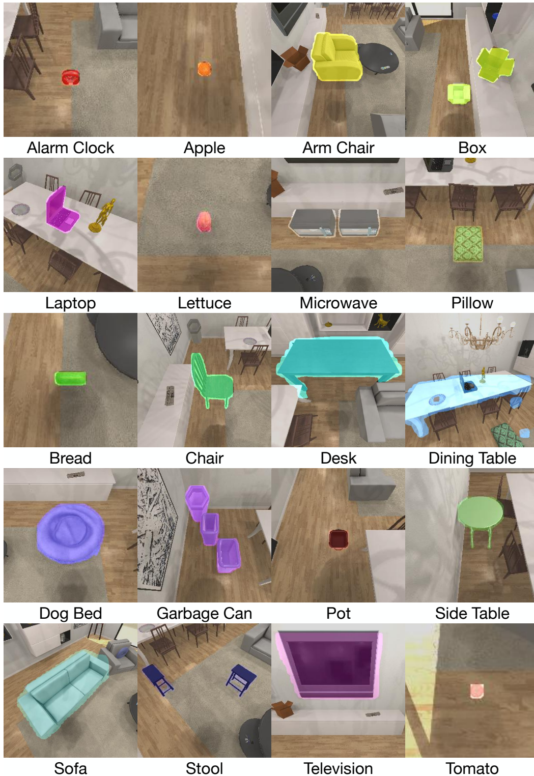
Figure 12: MaskRCNN's qualitative results on 20 used objects. We randomly spawn 20 objects in the testing scene LivingRoom227 and apply the pretrained MaskRCNN to obtain the segmentation results. The object prediction score is set to 0.5 and the segmentation probability is set to 0.1.
