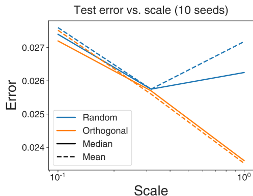
Figure 5. Test error for fully connected DEQs trained on MNIST. Learning rate tuning was performed for each initialization-scale pair, after which statistics were taken over 10 random seeds. Orthogonal initialization allows for larger initialization scales to train stably, and achieves lower test error.
