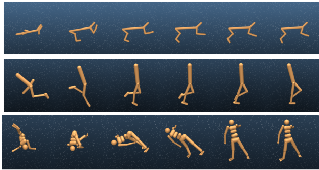
Figure 8. Noise to data paths computed with the trained CNFM on product manifolds representing robot’s state space: Cheetah (top), Walker (middle), and Humanoid (bottom).
