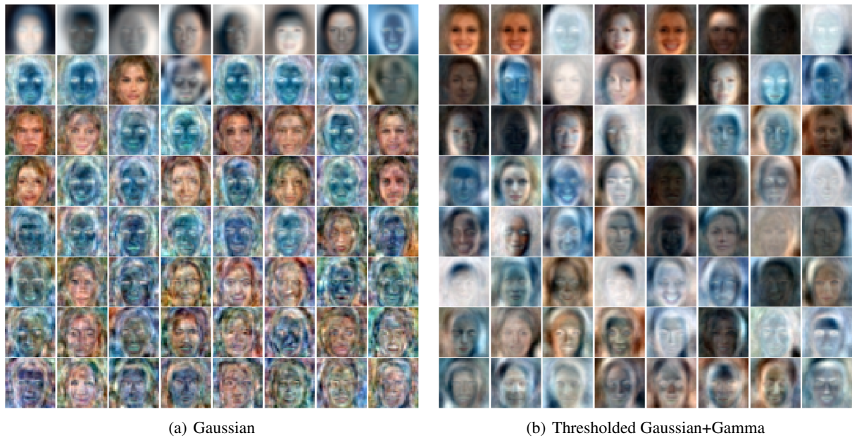
Figure 21. 512 dimensional latent space . Sampled entries from an estimated dictionary using an inference network trained with a DNN generator on CelebA. Entries are shown in descending order of Frobenius norm magnitude, with each row taking linearly spaced entries from the full dictionary. The sparse prior is set so to encourage 10% of latent features to be non-zero.
