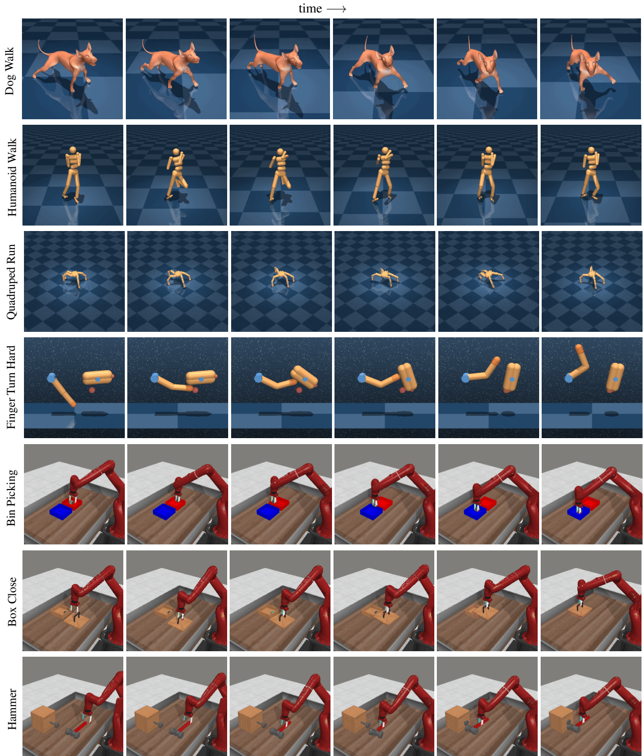
Figure 15. Visualizations. We visualize trajectories generated by our method on seven selected tasks from the two benchmarks, listed (from top to bottom) as follows: (1) Dog Walk, a challenging locomotion task that has a high-dimensional action space ( \mathcal{A} \in \mathbb{R}^{38} ); (2) Humanoid Walk, a challenging locomotion task ( \mathcal{A} \in \mathbb{R}^{21} ); (3) Quadruped Run, a four-legged locomotion task ( \mathcal{A} \in \mathbb{R}^{12} ); (4) Finger Turn Hard, a hard exploration task with sparse rewards; (5) Bin Picking, a 3-d pick-and-place task; (6) Box Close, a 3-d manipulation task; and lastly (7) Hammer, another 3d-manipulation task. In all seven trajectories, we display only key frames in the trajectory. Actual episode lengths are 1000 (DMControl) and 500 (Meta-World). Our method (TD-MPC) is capable of solving each of these tasks in less than 1M environment steps. Video results are available at https://nicklashansen.github.io/td-mpc .
