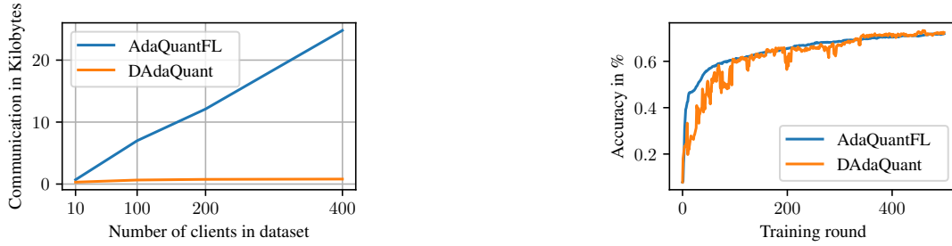
(a) Comparison of the per-round-communication for AdaQuantFL and DAdaQuant. We plot the average client→server communication per round that is required to train an MLR model on synthetic datasets with 10, 100, 200 and 400 clients. AdaQuantFL’s communication increases linearly with the number of clients because it trains the model on all clients at each round. In contrast, DAdaQuant’s communication does not change with the number of clients.
