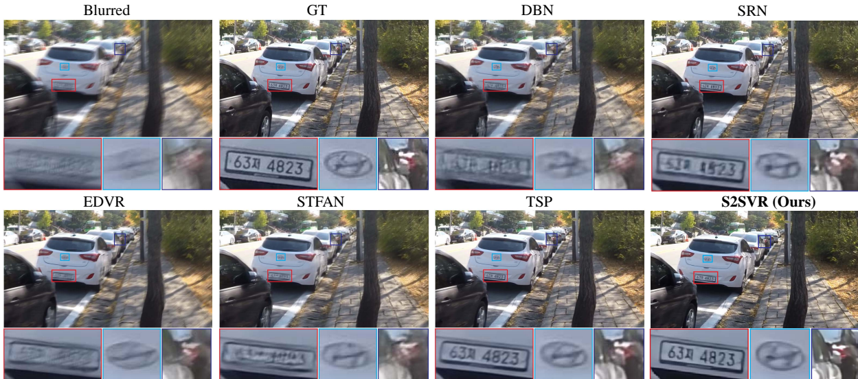
Figure 5. Visual comparison of video deblurring results on the GOPRO (Nah et al., 2017) dataset. Please zoom in for a better comparison.
