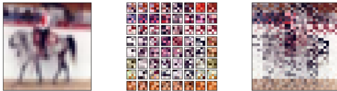
Figure 5. Example of Pixel Block Shuffle transformation (AprilPyone & Kiya, 2021a). An original CIFAR-10 image (left) is split into a grid of 4 \times 4 blocks of adjacent pixels, and the same random permutation is used to shuffle pixel positions within every block (middle). The transformed image is constructed by spatially concatenating the blocks according to their original positions in the grid (right).
