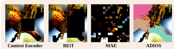
Figure 1. Self-supervised language, and vision, models learn representations by imputing data removed by masking. BERT : random word masks; Context encoder : random, fix-shaped mask; BEiT : random ‘blockwise’ masking; MAE : randomly mask out 75% of the image; ADIOS : multiple masks (N=3) generated by an adversarially trained masking model, post-processed with fully connected conditional random fields (Krähenbühl & Koltun, 2011).
