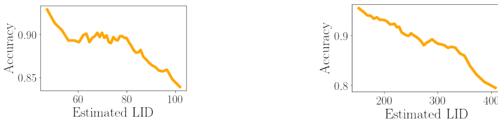
Figure 17: Average classifier accuracy per LID value on MNIST(left) and FMNIST(right) datasets. We can see a very strong negative correlation between those values.
