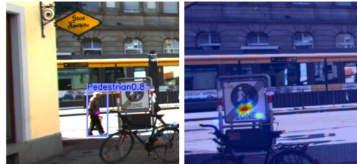
Figure 1. An example from the KITTI dataset with outputs of our method (object detection on the left and belief state on the right). We demonstrate that by fitting a Markov walk along an evolving spatial memory, a spatial belief state that codes object permanence emerges without explicit supervision.
