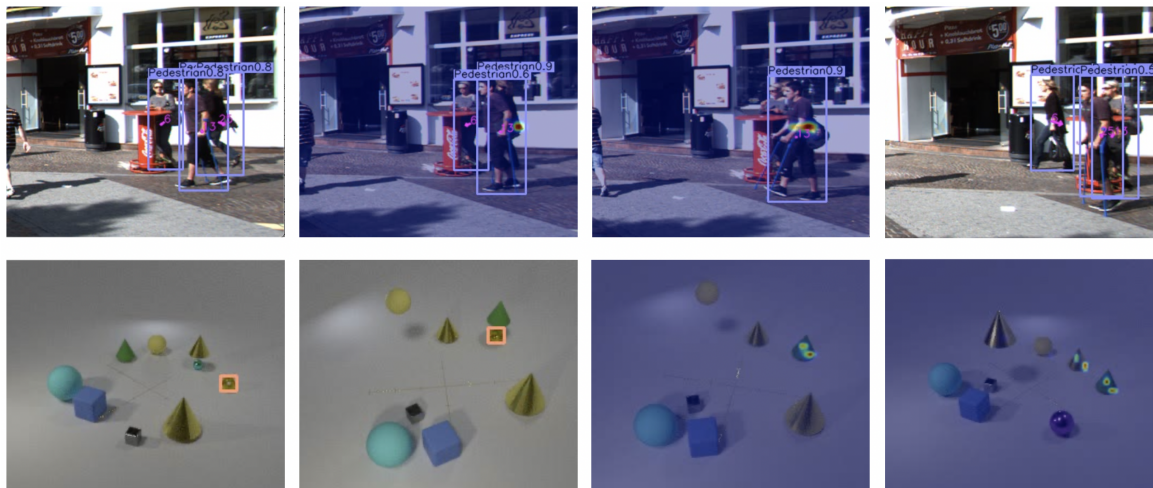
Figure 7. Failure modes of our approach on KITTI and LA-CATER-Moving (see link for full results). Model’s belief about the location of the invisible objects is visualized with a heatmap overlaid on the frames. Our method suffers from center overlap in the complex, three person occlusion and gets confused when two cones cover two spheres in the direct vicinity from each other.
