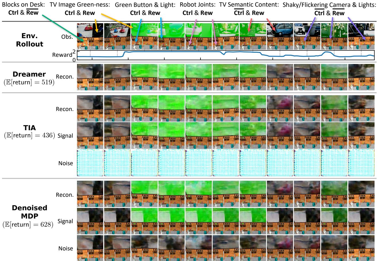
Figure 4: Visualization of learned models for RoboDesk by using decoders to reconstruct from encoded latents. For TIA and Denoised MDP, we visualize how they separate information as signal versus noise. In each row, what changes over frames is the information modeled by the corresponding latent component . E.g., in the bottom row, only the TV content, camera pose and lighting condition change, so Denoised MDP considers these factors as noises, while modelling the TV hue as signal. See our website for clearer video visualizations.
