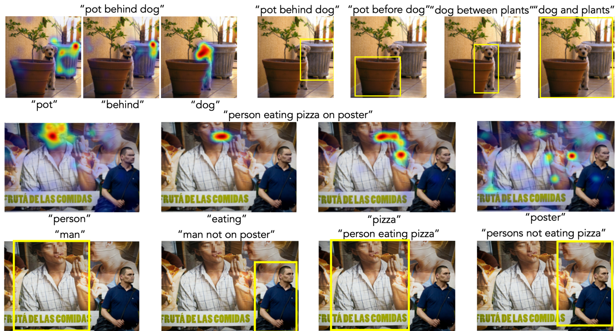
Figure 3. Grad-CAM visualization and bounding box prediction on unseen images. X-VLM predicts correct regions even though the textual descriptions only differ in a single word. X-VLM can also align each word in the text to the corresponding image region. Appendix A.4 gives more examples, showing X-VLM’s superior ability of multi-grained vision language alignments.
