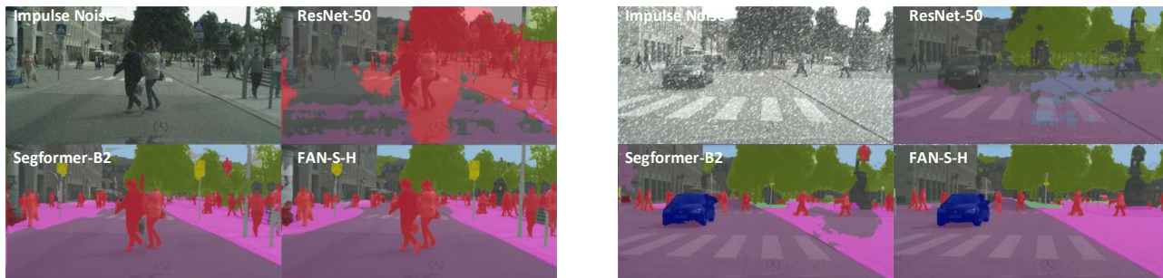
Figure 6. Segmentation visualization on corrupted images with impulse noise (severity 3) and snow (severity 3). We select the recent state-of-the-art SegFormer model (Xie et al., 2021) as a strong baseline. FAN-S-H denotes our hybrid model. Under comparable model size and computation, FAN achieve significantly improved segmentation results over ResNet-50 and SegFormer-B2 model. A video demo is available via external players and in Figure 8 in the appendix.
