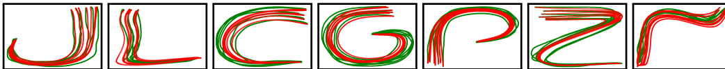
Figure 5: Imitating expert examples from the LASA dataset (Khansari-Zadeh and Billard, 2011). Reproduced motion in red and shown demonstration in green.
