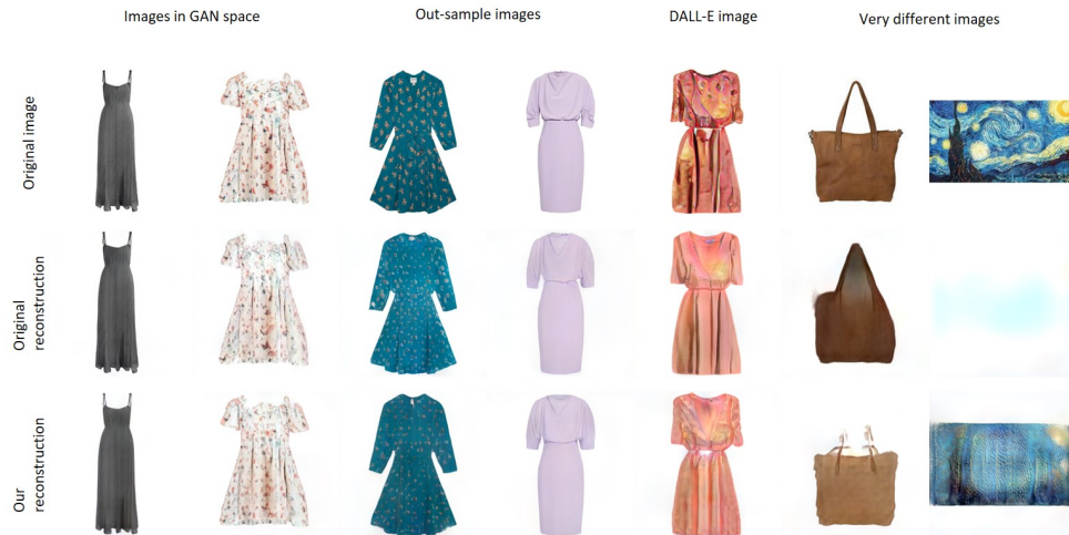
Figure 2: Example results of image embedding. The images in first row are the input images. The second row shows images found without using the pixel-level loss, and the third row shows images found using the pixel-level loss.
