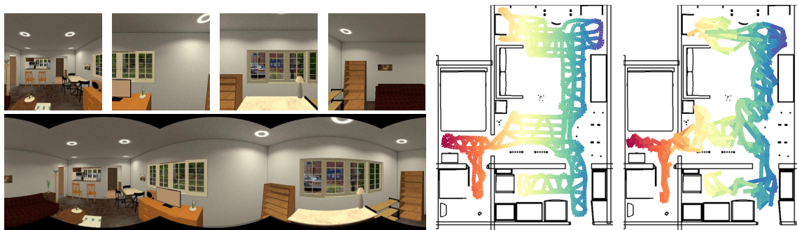
Figure 2: An example of the iGibson environment; (left) the quadruple-view at the location of observer and the constructed panorama image; (middle) a ground truth trajectory; (right) prediction
