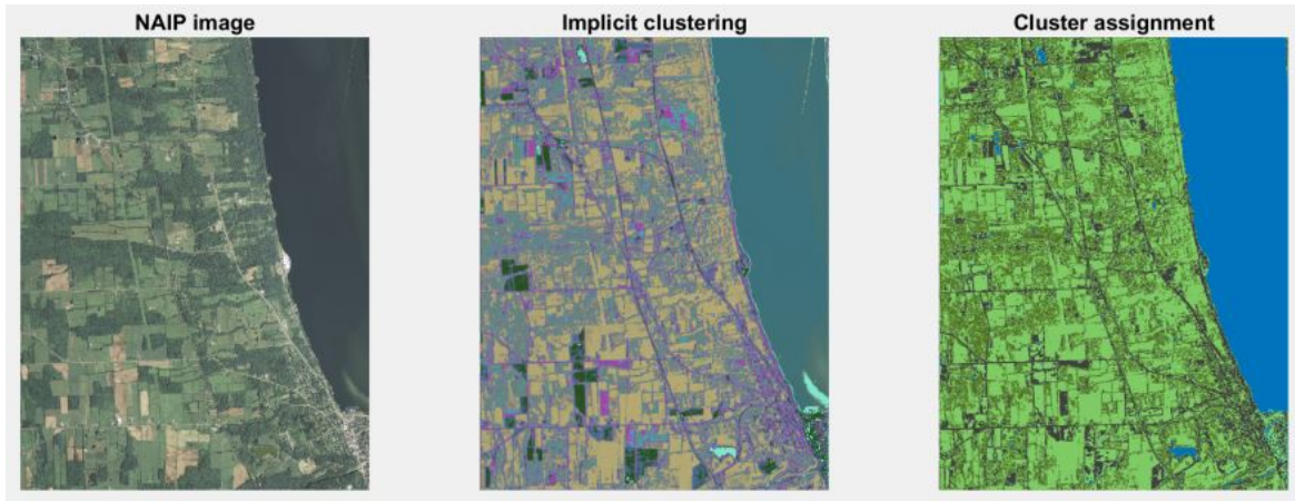
Figure F.1: Unsupervised clustering using implicit QR loss (middle) of a NAIP tile (left). On the right, we show the assignment of the 12 clusters to 4 land cover labels: water (blue), tall vegetation (darker green), low vegetation (lighter green) and impervious/barren (gray).
